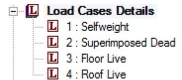
Figure 12.4-11: Basic load cases adopted in STAAD model.
