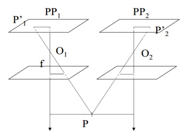
Position of P is uniquely determined by the intersection of lines  $P'_1O_1$  and  $P'_2O_2$
