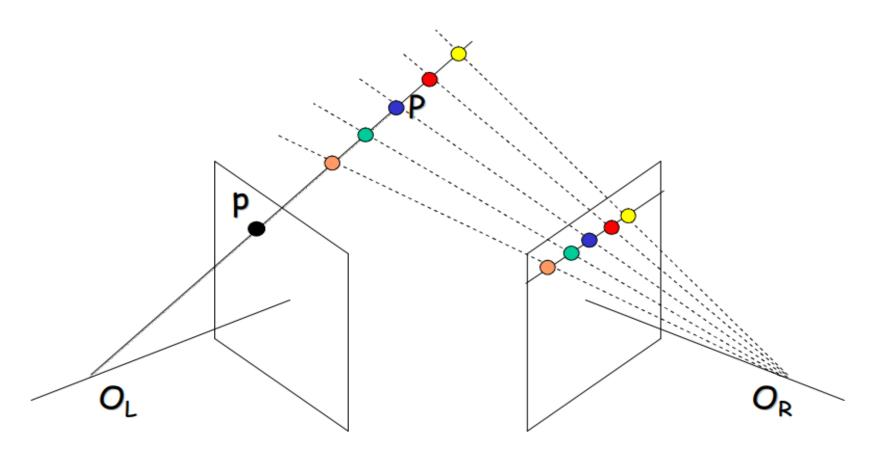
A second camera can resolve the ambiguity, enabling measurement of depth via triangulation.
