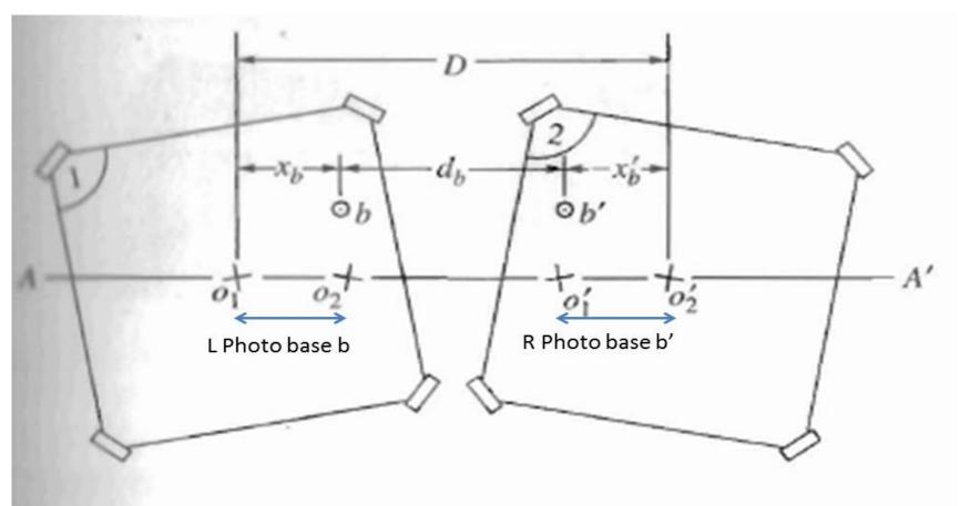
The image of each photo nadir, P.P in a vertical photo  $(o_1 \text{ and } o_2')$  appears on the other photo
