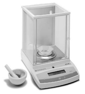
Fig. 2.1. Electronic analytical balance. (Courtesy of Denver Instrument Co. Denver Instrument Company owns all images.)
