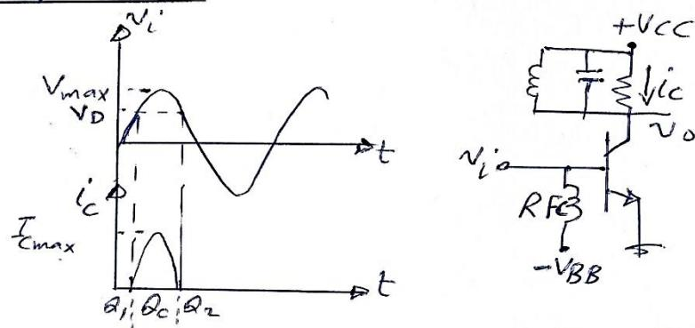
The amplifier conducts for angles less than  $180^\circ$ . This mode can have a great efficiency than Class B but it creates more distortion than class A or B amplifiers. This class is used in high frequency applications and high power. The RFC (Radio-Frequency Choke) has a high impedance at high frequency input and thereby prevents the dc source from shorting the ac input. The input must reach the level sufficient to overcome both the negative bias and \$V\_{BE}\$ drop.
