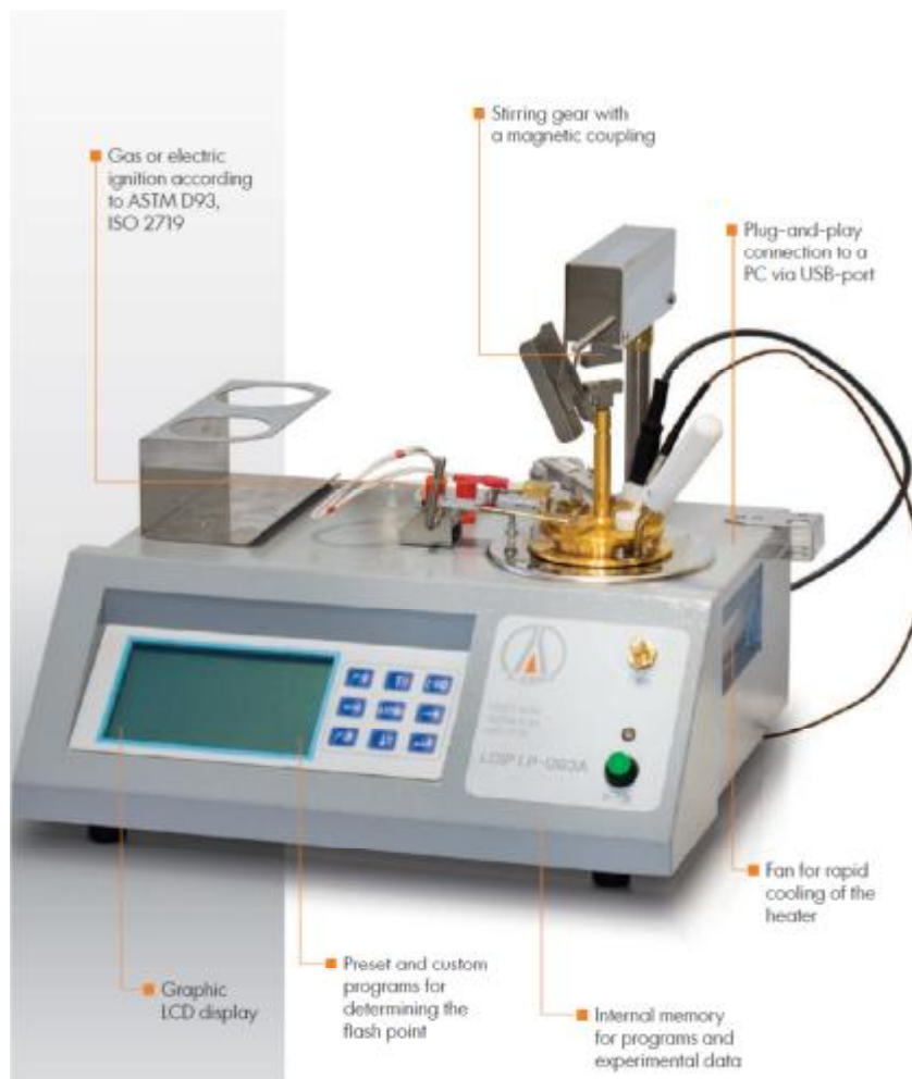
Pensky-Martens closed-up testing system
