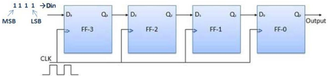
Let all the flip-flop be initially in the reset condition  $Q_3 = Q_2 = Q_1 = Q_0 = 0$ .
