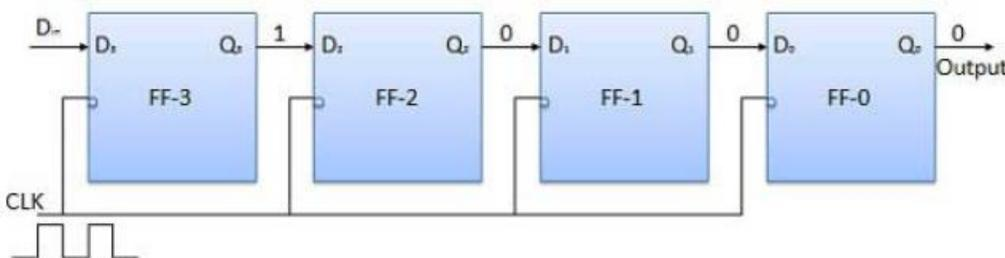
Apply the next bit to  $D_{in}$ . So  $D_{in} = 1$ . As soon as the next negative edge of the clock hits, FF-2 will set and the stored word change to  $Q_3 Q_2 Q_1 Q_0 = 1100$ .
