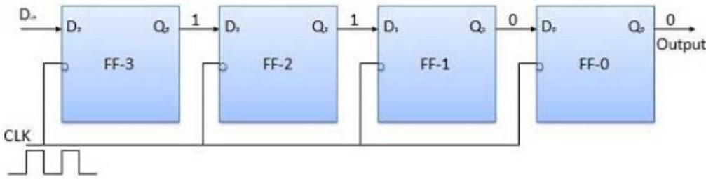
Apply the next bit to be stored 1 to  $D_{in}$ . Apply the clock pulse. As soon as the third negative clock edge hits, FF-1 will be set and output will be modified to  $Q_3 Q_2 Q_1 Q_0 = 1110$ .
