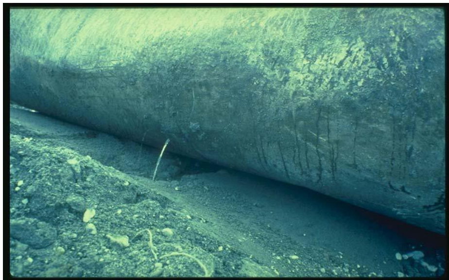
Oil spillage caused by fracture of pipelines.
