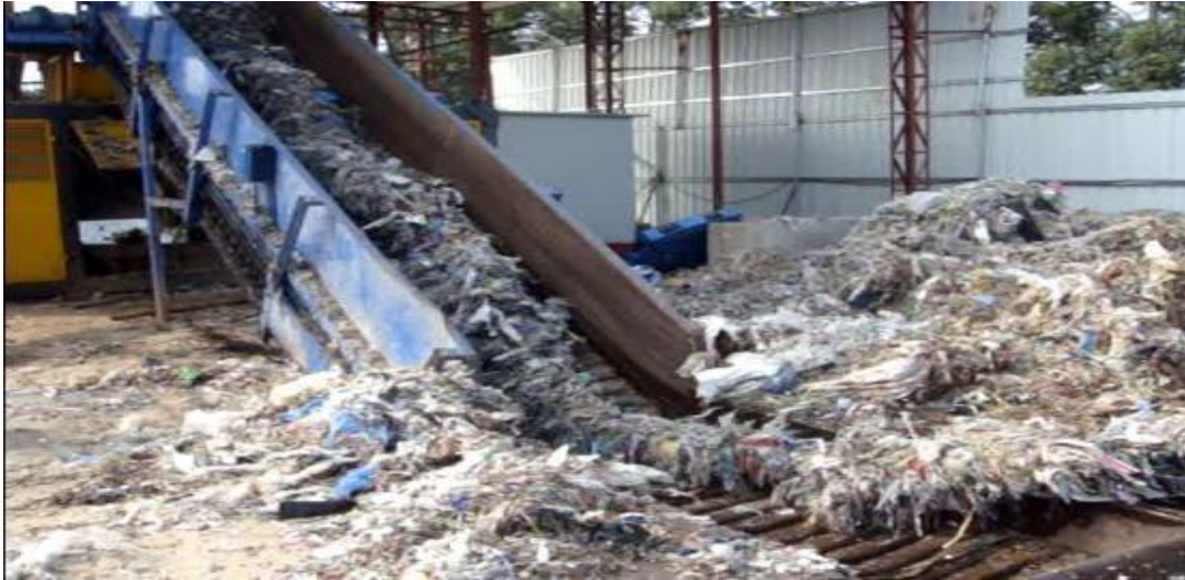
Fig. 4-3 Paper and Cardboard Shredding.
