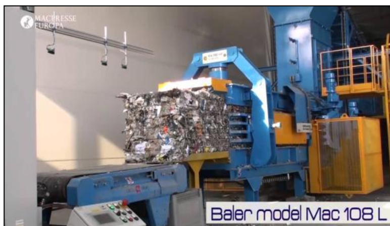
Fig. 4-2 Baler to Bale Plastics Paper, Cardboard and Aluminum Cans.
