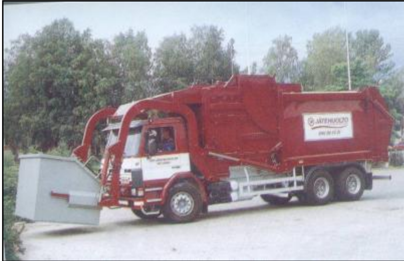
Fig. 8.1 Typical example of mechanically loaded collection vehicle used for the collection of residential wastes
