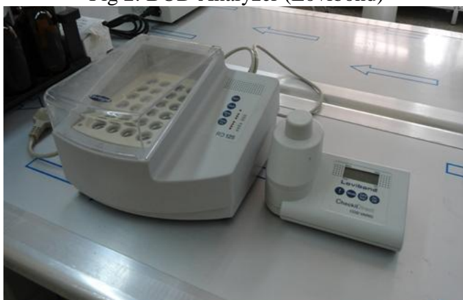
Fig 3: COD Analyzer with Thermo reactor
