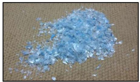
**Plate 1.** Sample of (PET- aggregate).
