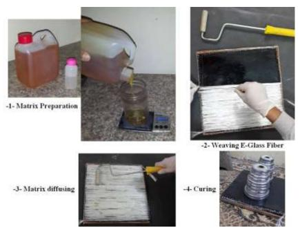
Figure 3. Specimen molding process
