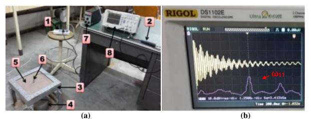
Figure 5. a)Free vibration test setup; (1) Power supply, (2) Impact hammar, (3) Testing structure, (4) weights, (5) Tested plate, (6) Accelerometer, (7) Charge amplifier for Accelerometer, (8) Oscilloscope; b) Generated response and FFT wave.
